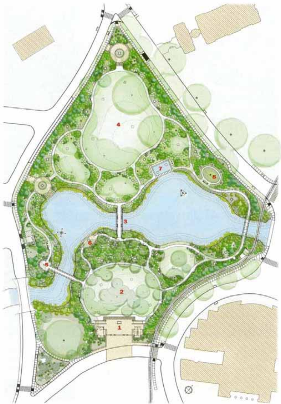
City Park roadways define the garden site. In the plan above, the New Orleans Museum of Art is at lower right, near the entry plaza (1). From the pine grove (2), a visual axis extends across a pedestrian bridge (3) and over the lagoon to the oak grove (4). Other features include an exedra (5), an overlook terrace (6), a cascade pool (7), and a sculpture theater (8). City Park's miniature scenic trains skirt the garden near the museum.
